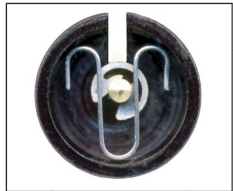
Be sure the V-shaped jet needle retaining clip is in place and will hold the jet needle securely in the slide.
